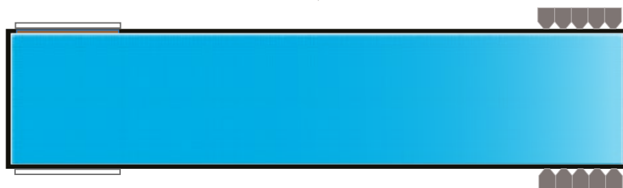
Figure 3: a tunnel ventilated house with fans at one end and inlets at the other end (on both sides).
